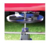
A standard output (red) tray featuring the EV-N-SPRED 3 hole drop mechanism with the DUAL port adjustable shut off system. This system applies all granular fertilisers evenly and efficiently in a 180 degree balanced spread pattern, saving time and money due to its true one pass even application.
